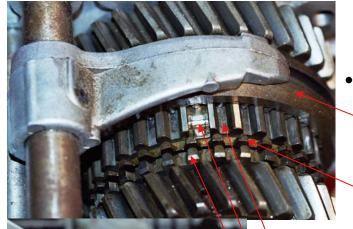
Spline (*synchronizer hub*) attached to input shaft
